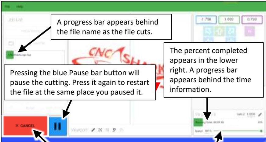
Pressing the CANCEL button will stop the machine movement. To restart the file press the Blue Run button. The file will restart at the beginning – not where it left off.
