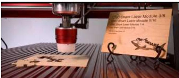
**Laser Module** (available with 2- or 7-watt power)\* Engraves in a variety of soft materials such as wood, paper, and leather. Also cuts thin materials\*\*.
