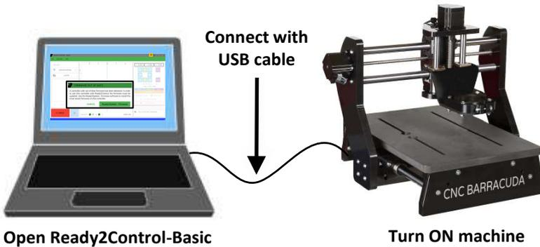
**4.1** Before you attempt to update the firmware on your machine's control box, make sure your computer is connected to the machine with the USB cable and the machine is turned on.
