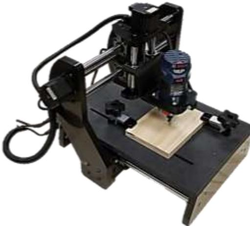
**4.3** Install the appropriate bit in the router and secure your project material to the table of your machine using the provided clamps and carriage bolts.
