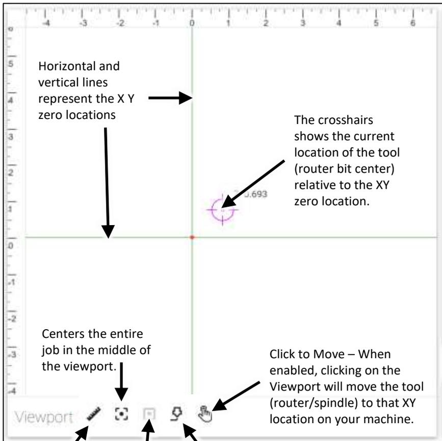
Horizontal and vertical lines represent the X Y zero locations
