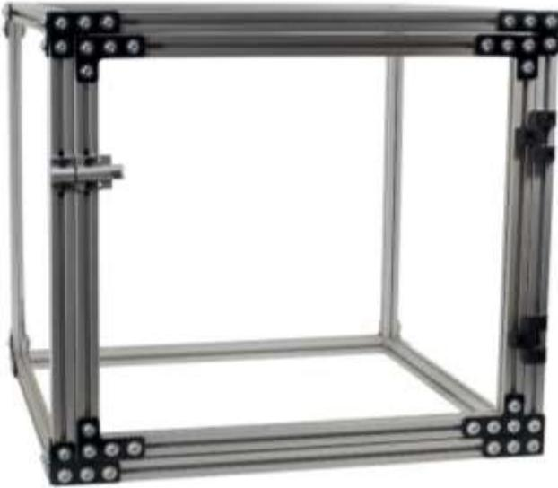
The **CNC machine enclosure** is designed to help control dust, add safety and reduce machining noise. Made with an aluminum frame, acrylic panels and steel connectors. Hinged access door with magnetic catch allows for easy material removal or bit changes. Pre-drilled 3" hole for cords allows for the case to be placed on any flat surface. Ships flat, assembly required.
