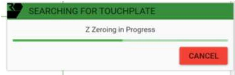
**Step 5** The Z axis will move down until the tip of the router bit touches the touchplate. It will then retract up to the Safe Z Height that was set in the control panel ([page 41](#)).
