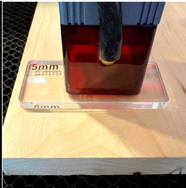
Image 26: Z Height Alignment
