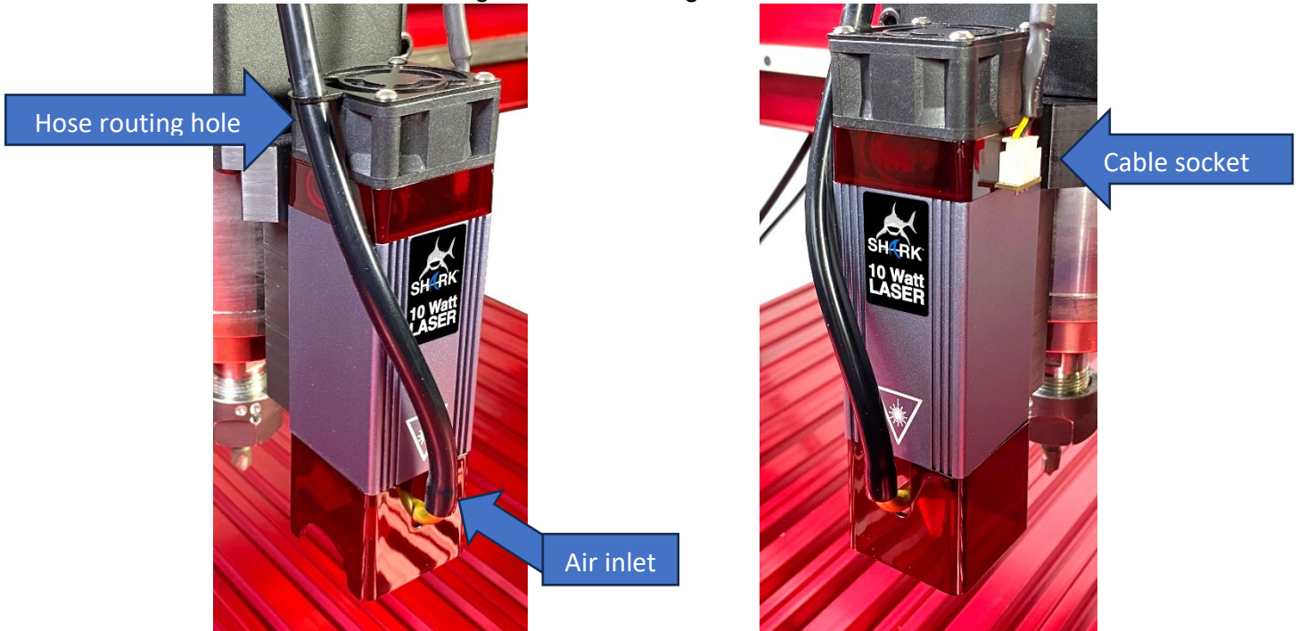
Image 6&7: Connecting Cable and Air Hose
