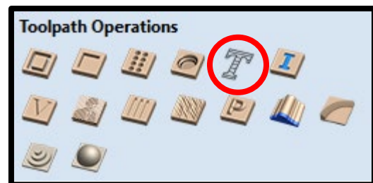
Image 22: Quick Engrave Toolpath
