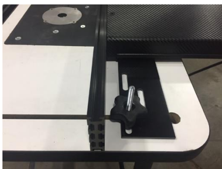
Figure 1 - R2R Fence Positioned 3" - 4" From Mounting Bracket
