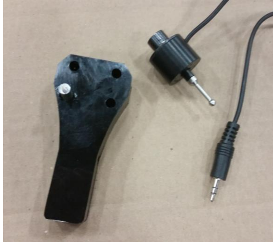
Touch probe and attachment arm
