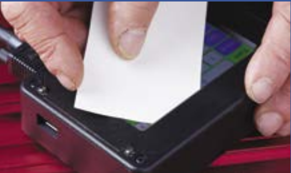
Wipe the Pendant screen with a soft cloth and remove sawdust buildup between the case and screen with a folded piece of paper.
