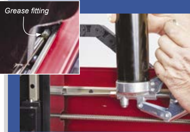
To lubricate the Z-axis bearings, you'll find the grease fittings behind the spindle mount.
