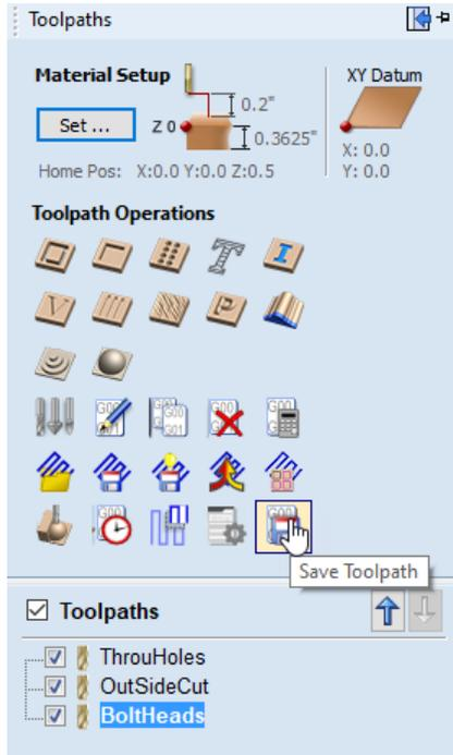
Since all the toolpaths use the same tool, we can run the G-Code in one file. The order is important and it's a good habit to get the stuff inside done before the cuts with the tabs. You can edit the order with the arrow tool pointed at by the big red arrow.
