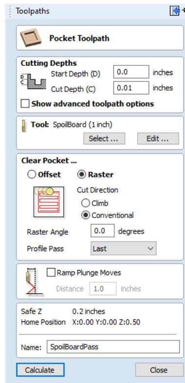
I call it the mowing the grass toolpath. Adjust the cut depth as necessary. Running this file multiple times is preferable to taking big swings to level the spoilboard.
