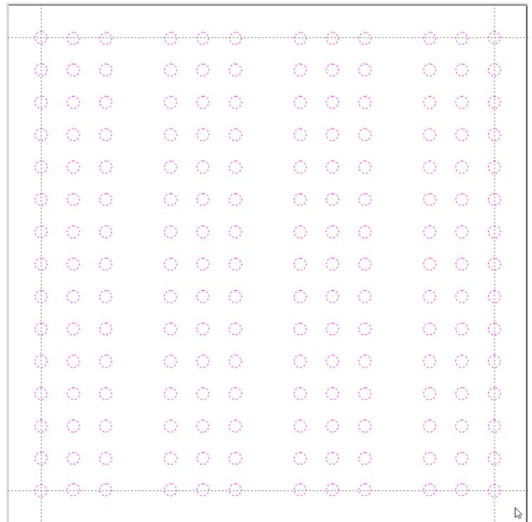
With all the thru holes selected, open the toolpaths tab and select the drill toolpath.
