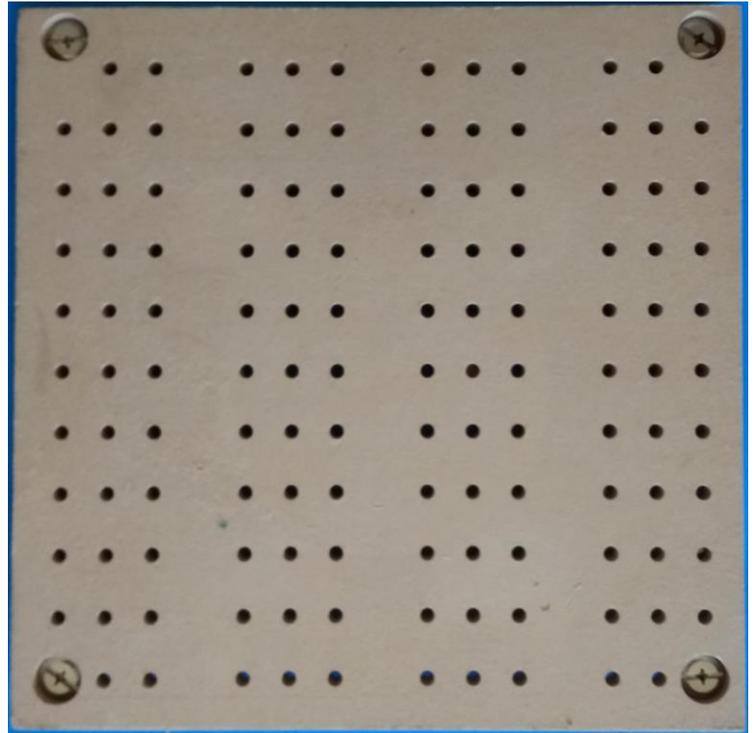
Spoil board prototype. This final project has the thru holes on  $\frac{3}{4}$ " spacing to match the t-track spacing. This one had 1" on the Y. Tighter spacing is better.
