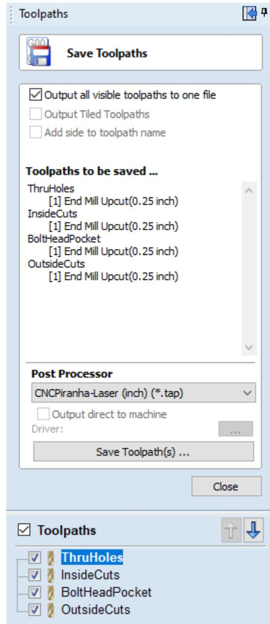
As always select the correct post processor and select the toolpath order as all these toolpaths can be cut at the same time. I like to go from inside to outside when using tabs.
