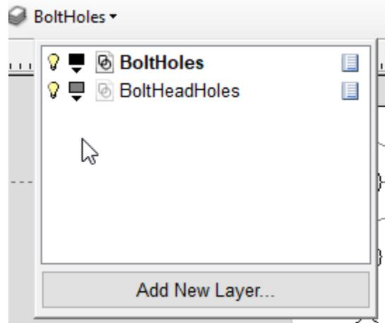
Click the light bulb next to the BoltHeadHoles to show just the thru holes that we will be drilling.
