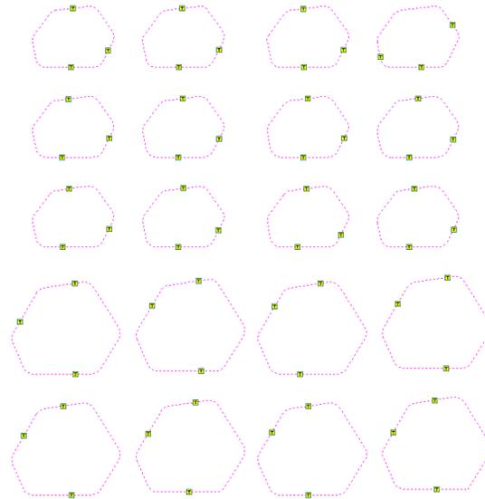
Select just the bolt head layer, select the bolt head circles and create a pocket toolpath for those.
