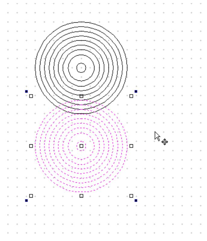
The inner two circles are for the bolt shaft and the bolt head. The others are the template so we can see just what the offset of the plates is in design. Move them to a new layer.
