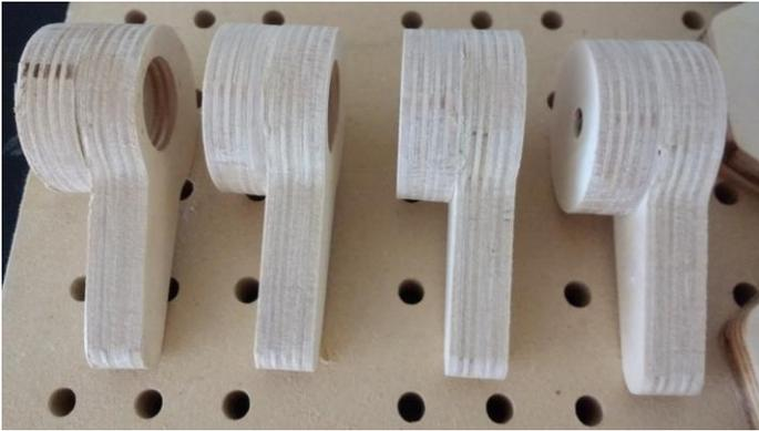
Cam levers are two pieces glued together. I used the bolts and oval nuts to clamp while drying. The levers keep the cam plates firmly to the spoil board.
