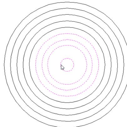
I will have four layers when done. The outside profile cut, the bolt head pocket, the thru hole, and the inside cut for the plate that is used with the cam layer.
