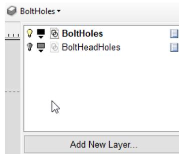
With all the bolt head pockets selected, open the toolpaths tab and select the pocket toolpath.
