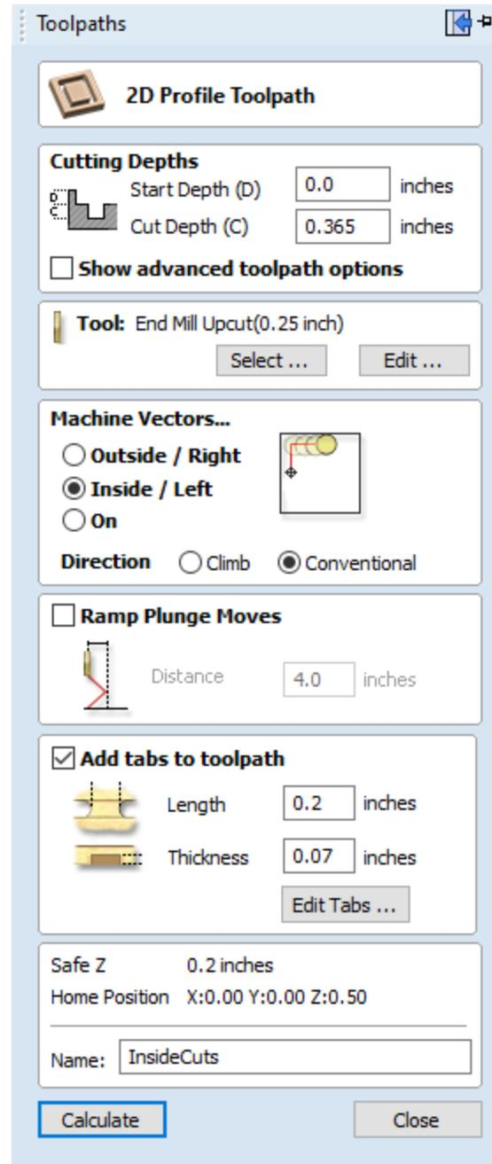
The last toolpath we need is the for the bolt shaft. Select hold the bolt shaft layer and select those circles.
