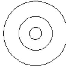
Then we need to more circles on the same center point of .28 (a little larger than the bolt shaft) and one a little larger .78 than the bolt head.
