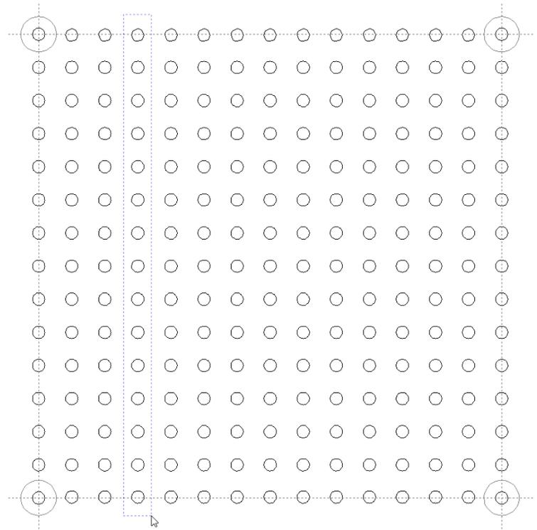
Copy and paste a part of a row between the corner bolt head holes.
