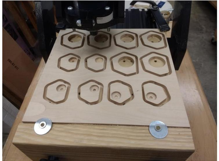
Cutting the original prototype plates using the maximum cutting area of the Piranha.
