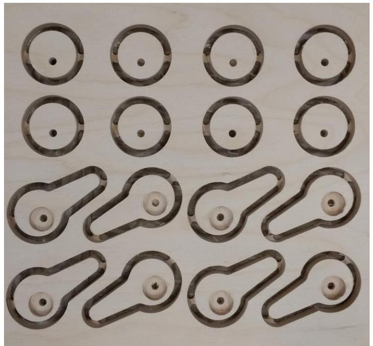
The original prototype levers and plates. Notice that they are not mirrored with right and left pivot points. In these production CAM files they are and will add more versatility.
