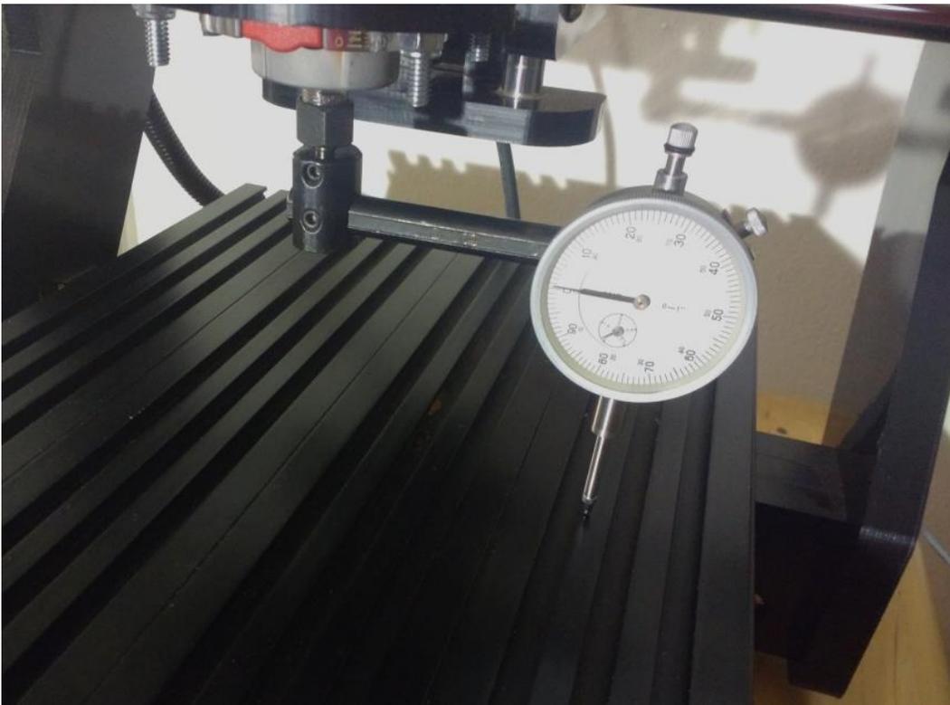
A fly cutter with an inexpensive dial gauge makes a good way to tram your router for perfect cuts. When you surface the spoil board, if you have a scallop pattern, you might want to get some shim material and tune the routers mounting.
