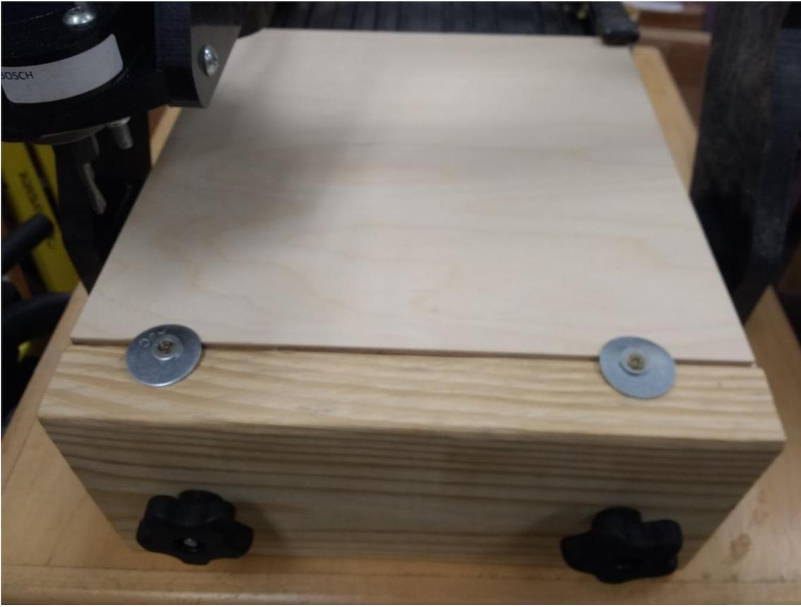
Another quick way for a low-profile hold down while cutting a spoil board to the front of the T-Track.
