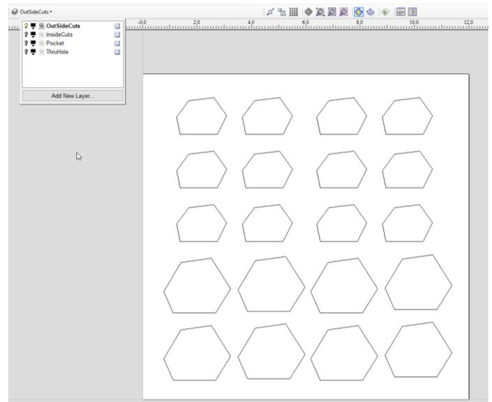
Select the Profile Toolpath operation from the Tool Path tab and set the desired settings for the outside cuts.
