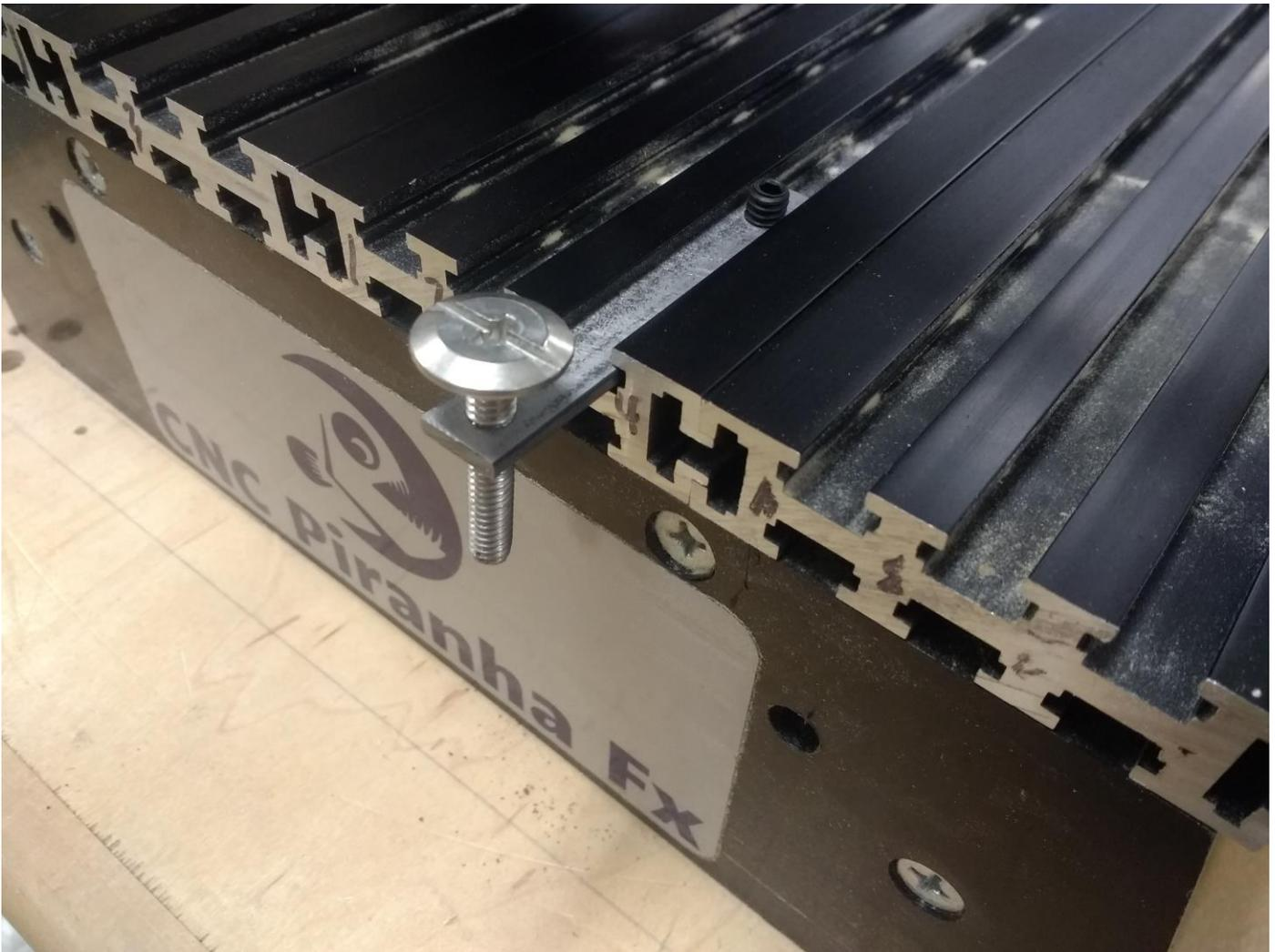
A piece of flat bar also can become a handy clamp on the Piranha to cut to the front of the bed.
