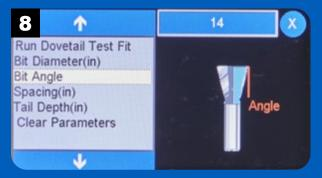
Select Bit Angle to set the parameter for the angle of the router bit. You can usually find this information on the product packaging.
