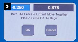
Press OK to move the fence and lift to the starting position for cutting the dovetail socket.
