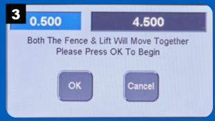
Press OK to move the lift and fence to the starting position to finish routing the pins.
