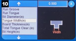
Setting the tongue width determines how much material to remove from each edge to form a tongue.
