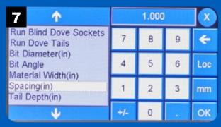
Set the spacing between tails by entering the value and pressing OK.
