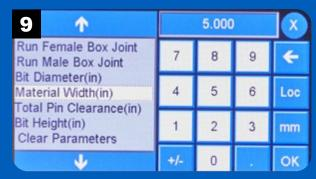
Enter the width of the workpiece and press OK.
