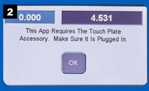
The value field in the upper right displays the current value for the position of the router lift. Install the touch plate and press OK to continue.
