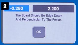
Clamp the workpiece to the miter gauge with the end against the router tabletop and the back edge against the router table fence. Press OK to continue.
