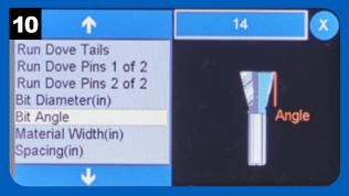
Select Bit Angle to set the parameter for the angle of the router bit. You can usually find this information on the product packaging.
