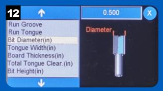
Use a straight bit for routing tongues. Use the Bit Diameter function to set the bit's diameter.
