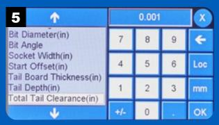
Enter the value for the Total Tail Clearance and press OK. NOTE: The value entered will be applied to each side of the dovetail.
