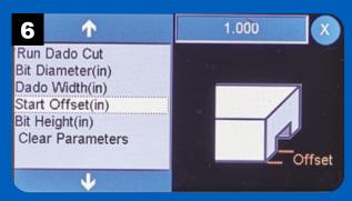
Use the Start Offset function to set the distance of the edge of the dado from the edge of the workpiece.
