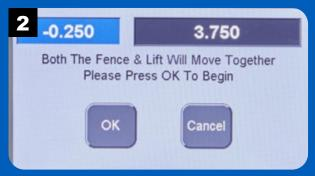
Press OK to move the fence and lift into their starting positions
