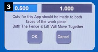
To create the dovetail, each side of the workpiece must be routed. Press OK to move the fence and lift to the starting position.
