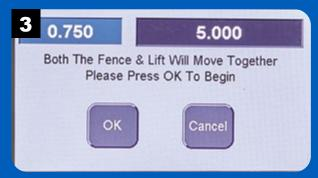
Pressing OK will move the router fence and lift to the starting position for routing the dado. The fence will move multiple times until the entire width of the dado is complete.
