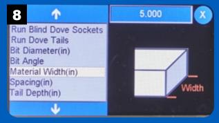
Enter the overall width of the material you're using to create the half-blind dovetail joints by pressing the value field.
