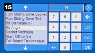
Enter the angle of the dovetail and press OK.
