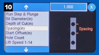
Create evenly spaced dowel holes by using the Spacing function to set the center-to-center distance between dowel holes.
