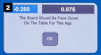
Place the workpiece face down on the router table.
