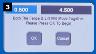
Press OK to move the lift and fence to the starting position to cut a dovetail.
