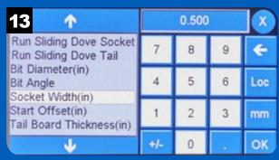
Enter the desired width for the dovetail socket and press OK.
