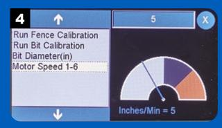
Change the speed range of the motors that control the fence and router lift by selecting Motor Speed from the menu.
