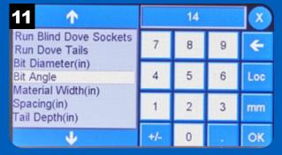
Enter the angle of the dovetail and press OK.
