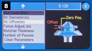
Using the illustration on the screen, measure the Bit Offset.
