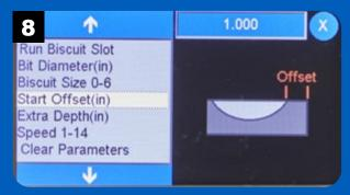
The Start Offset option sets the distance of the end of the biscuit slot from the edge of the workpiece. Press the value button to change this distance.
