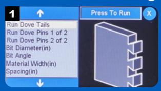
Run Dove Tails runs the app to create the dovetails on the tail boards.
