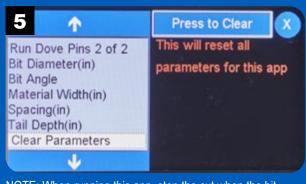
NOTE: When running this app, stop the cut when the bit reaches the baseline (or bottom) of the pins.
