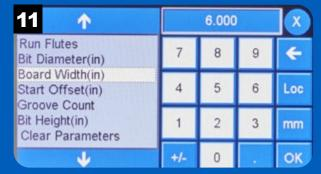
Enter the width of the workpiece and press OK.
