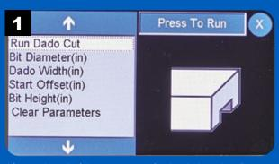
After setting all of the parameters for the dado, select Run Dado Cuts then Press to Run.
