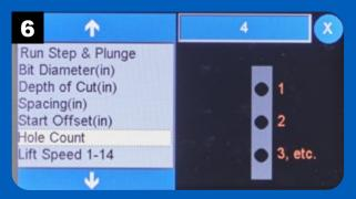
Set the number of dowel holes using the Hole Count function.
