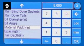
Enter the width of the workpieces and press OK.
