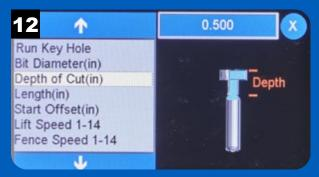
The Depth of Cut option sets the overall depth of the key hole slot in the workpiece.
