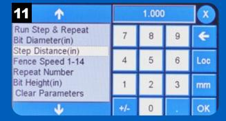
Enter the desired distance for the step distance and press OK.
