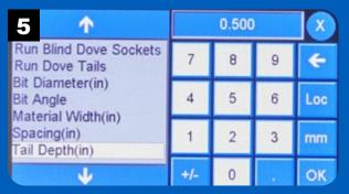
Enter the tail depth and press OK. To accept the default value displayed, press OK without entering a value.
