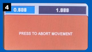
As the router lift and fence move, you can press the red button to abort the movement if necessary. Otherwise, the fence and lift continue to move to the starting position.
