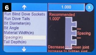
The Spacing parameter sets the center-to-center distance between the dovetails. Note the recommended spacing parameters and tips on the screen.
