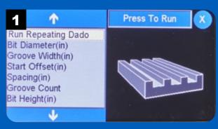
After setting all of the parameters for the dado, select Run Repeating Dado then Press To Run.
