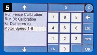
On the numeric keypad, enter a value for the motor speed (1=slow, 6=fast) then press OK.
