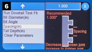
The Spacing option sets the distance between the dovetails. Note the tips and recommendations on the screen.
