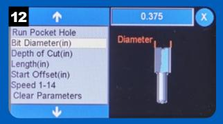
The diameter of the router bit determines the width of the pocket hole. Select Bit Diameter to change this value.
