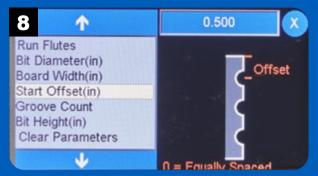
The Start Offset option sets the distance of the centerline of the first flute from the edge of the workpiece. NOTE: Entering a zero value spaces the flutes evenly across the widht.
