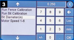
On the numeric keypad, enter the diameter of the router bit installed in the router and press  $\mathsf{OK}.$
