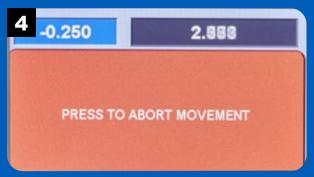
During fence and lift movement, you have the option to abort the operation.
