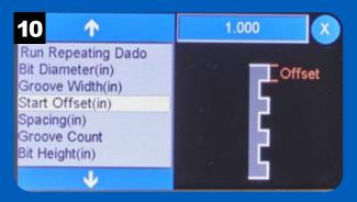
Use the Start Offset function to set the distance of the edge of the first dado from the edge of the workpiece.
