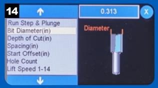
Use the Bit Diameter function to set the diameter of the router bit. The dowel hole diameter will match the bit diameter.
