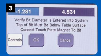
Make sure the router bit is below the surface of the table and press OK. The Controls button allows you to make adjustments in the fence and lift position before continuing.
