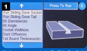
After the parameters are set, select Run Sliding Dove Socket.
