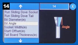
The Bit Angle is the angle of the dovetail router bit. This value can usually be found on the product packaging for the bit.
