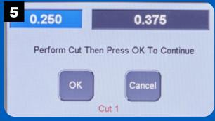
With the edge of the workpiece resting on the router table and the face against the fence, make the first pass. Press OK then rotate the workpiece 180° to make the second cut.
