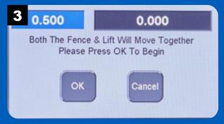
After pressing OK, the lift and fence will move to the starting position for routing the dovetails.
