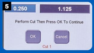
Make the first pass over the router bit then press OK. The fence will move to the next position. Repeat until the full width of the dado is complete.
