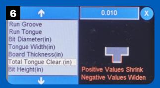
To create a joint with a snug fit without being too tight, finetune the tongue width by choosing the Total Tongue Clearance parameter.
