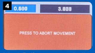
As the router lift and fence move, you can press the red button to abort the movement if necessary. Otherwise, the fence and lift continue to move to the starting position.
