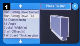
Select Run Sliding Dove Tail to begin routing the dovetail.
