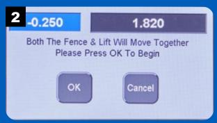
A message appears notifying you that the fence and lift will move when you press OK. Make sure the workpiece is tight against the fence before proceeding.
