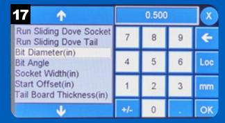
Enter the measured diameter of the router bit and press OK.
