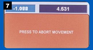
The router lift moves until it contacts the touch plate and displays the position in the upper right value field.
