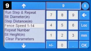
Enter a value from 1 (slow) to 14 (fast) for the fence speed and press OK.
