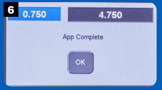
When all of the cuts are completed, the app stops. Reorient the workpiece to cut the other end and press OK to continue.
