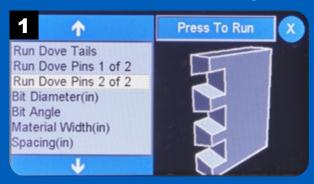
Still leaving the dovetail bit in place, press Run Dove Pins 2 of 2. This operation creates the angled sides of the pins to mate with the dovetails.
