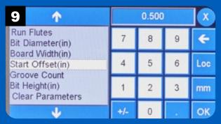
Enter the desired distance for the offset and press OK.
