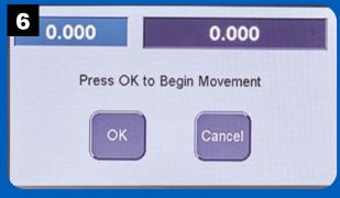
Pressing OK begins movement of the fence and touch plate toward the router bit.
