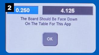
Place the workpiece facedown and press OK. NOTE: This operation requires a stop block on the fence. Refer to this video for details: {ADD LINK HERE}
