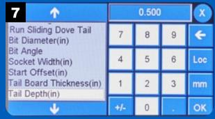
Enter the desired value for the depth of the dovetail and press
