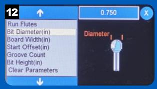
Set the bit diameter by pressing the value field in the upper right.
