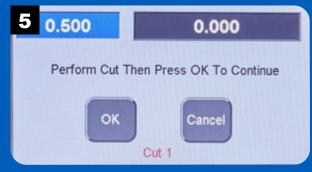
With the workpiece tight against the fence and table, make a pass to form one side of the tongue. Rotate the workpiece and make another pass to complete the dovetail. Press OK.
