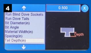
The Tail Depth is one parameter that controls the fit of the final half-blind dovetail joint. Note the recommended values and tips on the screen.
