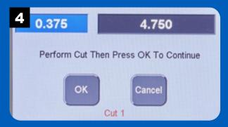
With the workpiece tight against the fence, make the first pass. Press OK. The fence will move to the next step position.
