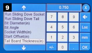
Enter the thickness of the workpiece and press OK.
