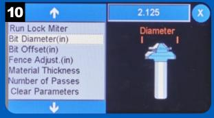
Use the Bit Diameter option to enter the largest diameter of the lock miter router bit. Use a set of calipers to obtain an accurate measurement.
