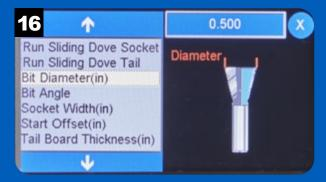
Set the bit diameter by pressing the value field in the upper right. **NOTE:** It's best to measure the actual diameter of the bit with calipers rather than rely on the stated diameter.
