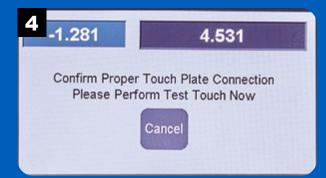
Tap the touch plate to the router bit to confirm that the plate is installed and connected correctly.
