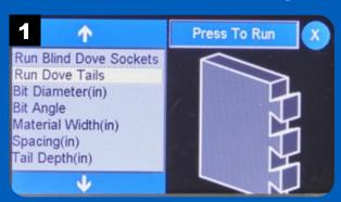
Select Run Dove Tails to rout the pins, or tails, that fit into the sockets you routed earlier.
