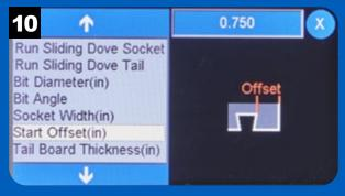
Choose the Start Offset function to set the distance of the socket edge from the edge of the workpiece.
