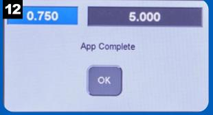
When all of the cuts are completed, the app stops. Reorient the workpiece to cut the other end and press OK to continue. Test the fit of the joint and tweak the parameters for a good fit.
