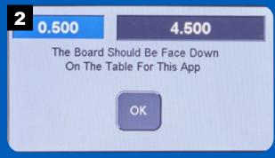
Remove the miter gauge and place the workpiece face down on the router table. Press OK.
