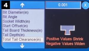
Press the down arrow to access other parameters for sliding dovetail joints. The Total Tail Clearance sets the amount of material to be removed from the width of the dovetail.
