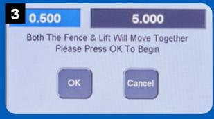
The fence and lift move to the starting position after pressing OK
