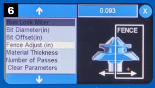
The Fence Adjust value allows you to fine-tune the fit of the lock miter joint. It's helpful to test the fit on scrap pieces the same thickness as the final workpieces.
