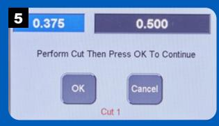
With the edge of the workpiece against the fence, make the cut to create the first flute. Press OK to move the fence to cut the second flute.
