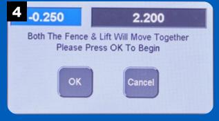
Press OK to use the same parameters to repeat the slotcutting operation on another workpiece or the opposite end of the workpiece.
