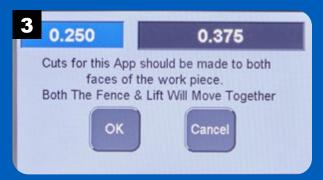
To create a tongue centered on the edge of the workpiece, you'll make a pass on opposite sides of the workpiece. Press OK to move the fence and lift to their start positions.
