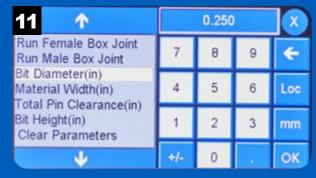
Enter the measured bit diameter using the numeric keypad then press OK.
