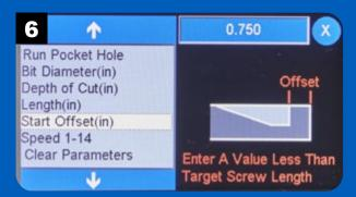
The Start Offset function sets the distance of the end of the pocket hole from the edge of the workpiece. This is determined by the screw length to be used.
