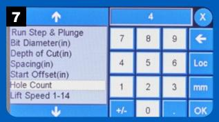
Enter the desired number of dowel holes to be routed and press OK.
