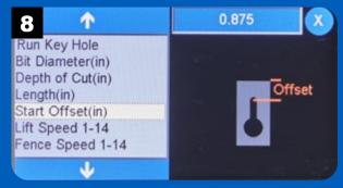
Use the Start Offset option to set the distance of the end of the slot from the edge of the workpiece.
