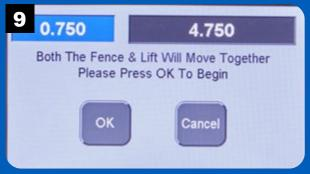
Pressing OK will move the fence and the lift to the starting position for cutting the female box joints. Ensure there are no obstructions on the router table and press OK.
