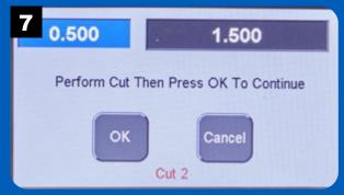
Repeat until all the sockets are cut on the end of the workpiece. After the last socket is routed, the app will stop.
