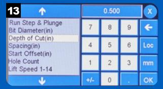
Enter the dowel hole depth and press OK.
