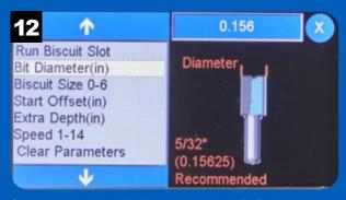
Start by entering the bit diameter using the Bit Diameter function. A 5½" bit is recommended. Press the value button in the upper right to enter the bit diameter.
