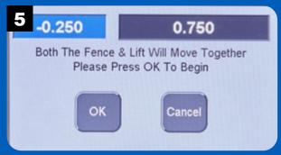
With the workpiece in place, press OK to start routing the dowel holes.
