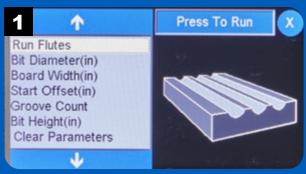
With the parameters set, press Run Flutes then Press To Run to start the app.
