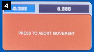
While the fence and lift are moving, you can abort the operation, if needed.
