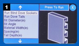
Select Run Blind Dove Sockets to begin cutting the sockets in the ends of the workpieces.
