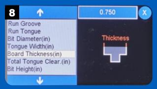
Use Board Thickness to set the thickness of the workpiece.
