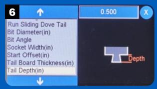
The Tail Depth option sets the length (depth) of the dovetail.
