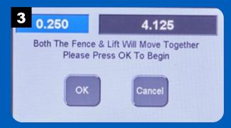
Pressing OK will move the router fence and lift to the starting position for routing the sockets. The fence will move multiple times until all of the sockets are routed.
