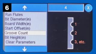
Specify the number of grooves to rout using the Groove Count option.
