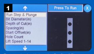
To start routing dowel holes, select Run Step & Plunge.
