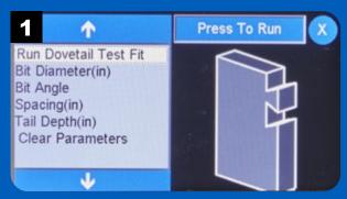
After setting the parameters, press Run Dovetail Test Fit to start the app. Select Press To Run to start.
