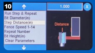
The Step Distance sets the distance of the fence from the centerline of the router bit.
