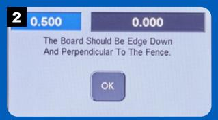
Clamp the workpiece to the miter gauge with one face against the miter gauge, one edge against the fence, and the end tight to the router table. Press OK to continue.
