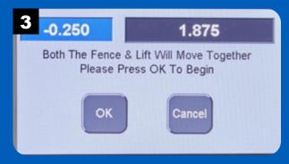
After pressing OK, the fence and lift will move to the starting position to cut the pocket hole.
