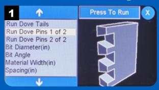
Leave the dovetail bit installed and select Run Dove Pins to make the first pass that removes the bulk of the waste between the pins.
