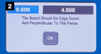
Clamp the workpiece to the miter fence with the end against the table and the edge against the fence. Press OK to continue.
