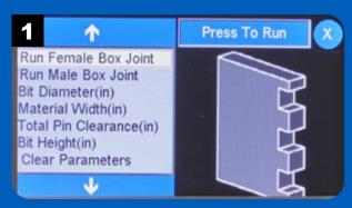
The function Run Female Box Joint cuts the spaces, or sockets, between the pins. Select Press To Run to continue.
