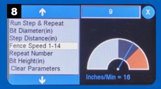
During the Step & Repeat app, the fence moves between each pass to set the distance for the next cut. The Fence Speed parameter allows you to control the speed.
