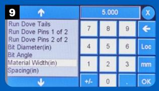
Enter the workpiece width and press OK.
