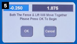
With the workpiece in position, press OK to start routing. The lift will raise and the fence will move forward then back. Keep the edge of the workpiece against the fence.
