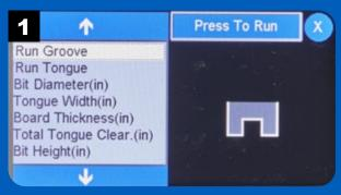
The Run Groove app routs the groove centered on the edge of the workpiece. Use a bit diameter the same width as the groove or smaller. Multiple passes create the desired width.
