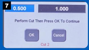
Repeat yntil all the tails are cut on the end of the workpiece. After the last tail is routed, the app will stop.
