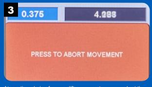
At any time during fence or lift movement, you can abort the operation.
