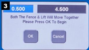
Pressing OK moves the router fence and lift to the starting position for routing the tails. The fence moves multiple times until all of the tails are routed.
