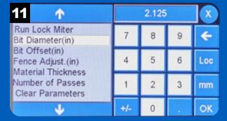
Enter the router bit diameter and press OK.
