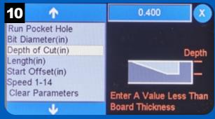
The Depth of Cut option sets the depth of the pocket hole at its deepest point. The value must be less than the thickness of the workpiece and may require some test cuts to refine it.
