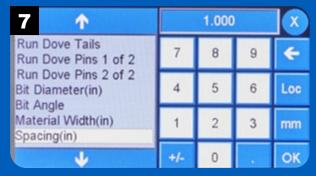
Enter the value for the desired spacing and press OK.
