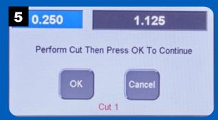
Make the first pass over the router bit then press OK. The fence will move to the next position. Repeat until the full width of the dado is complete.
