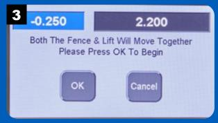
Pressing OK will move the fence and the lift to the starting position for cutting the female box joints. Ensure there are no obstructions on the router table and press OK.
