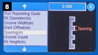
The Spacing function determines the edge-to-edge distance between the dados or grooves.
