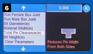
The Total Pin Clearance value reduces the pin width by subtracting the clearance value from each side of the pin.
