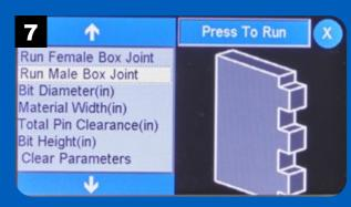
Cutting the male portion (pins) of the box joints follows the same process as cutting the female portion. Press Run Male Box Joint then Press To Run to continue.
