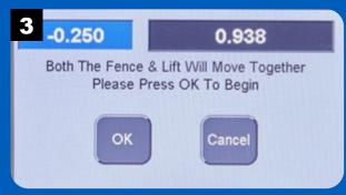
Press OK to reposition the fence and lift at the starting position for routing the dowel holes.
