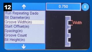
Select Groove Widths to set the overall width of the dadoes or grooves.
