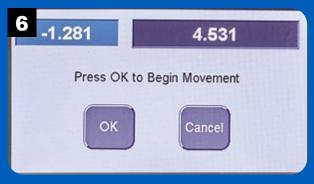
Ensure that the touch plate is flat on the table over the router bit and press OK.
