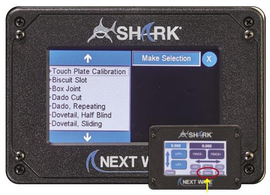
**Apps Menu Screen:** Press the Apps button on the Main Control screen to open the Apps screen. The Apps menu contains options for controlling specific **RS1000 Pro** functions. Press a menu item to open the setup screen for that option. To return to the Main Control Screen, press X in the upper right corner.
