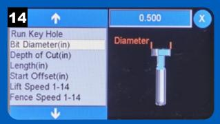
Select Bit Diameter to enter the diameter of the key hole router bit at its largest diameter.
