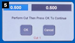
Make the first pass over the bit and press OK. Repeat this process until the app finishes.
