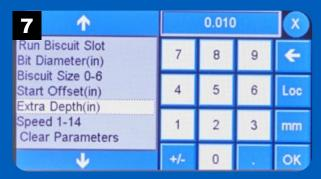
Enter the extra depth distance using the keypad then press OK.
