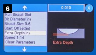
The Extra Depth option allows you to add space around the biscuit for glue relief and ease of assembly. Press the value button in the upper right to assign this distance.
