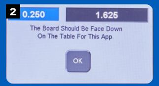
Place the workpiece face down (where the dadoes are to be cut). Press OK to continue.
