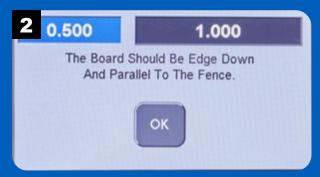
Place the workpiece vertically with one edge against the router table and one face against the fence and press OK.
