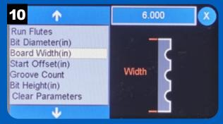
Press Board Width to enter the overall width of the workpiece by pressing the value button on the upper right.
