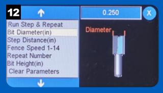
Set the diameter of the installed router bit using the Bit Diameter parameter.
