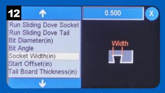
Select Socket Width to set the width of the dovetail socket. If this value is greater than the bit diameter, the *RS1000 Pro* will adjust the fence position to rout the socket in multiple passes.
