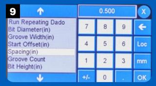
Enter the desired spacing between dadoes and press OK.
