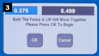
The fence and lift move into the starting position after pressing OK.
