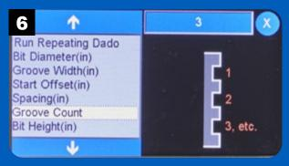
Select Groove Count to set the number of dadoes or grooves to cut in the workpiece.
