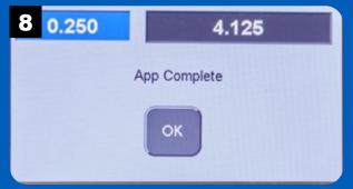
When all of the dadoes or grooves have been cut to their desired width and spacing, the app stops automatically. Press OK to exit.
