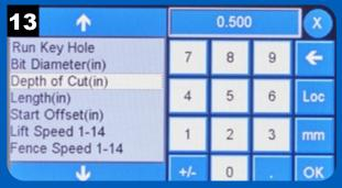
Enter the desired depth of the key hole and press OK.
