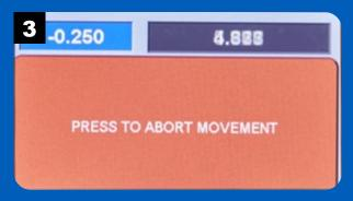
The fence and router lift both move automatically to create the slot with the preset dimensions. Press the red area to abort movement if necessary.
