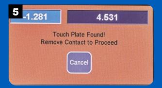
The red screen confirms a proper touch plate connection.
