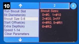
Next, set the size of the biscuit slot by selecting a conventional biscuit size using the Biscuit Size function. Press the value button in the upper right to change the biscuit size.
