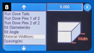
Set the parameter for the width of the workpieces by selecting Material Width.
