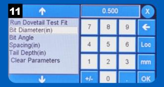
Enter the measured bit diameter and press OK.
