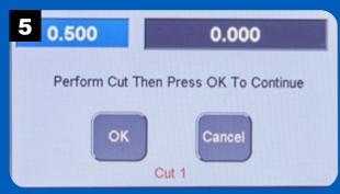
Make the first pass and press OK. Repeat the process until all of the dovetails are routed.
