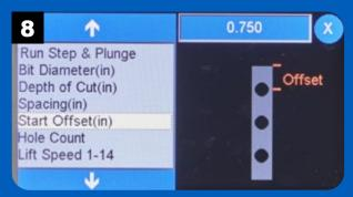
To establish a predetermined distance from the edge of the workpiece for the first hole, use the Start Offset function.
