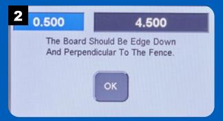
Clamp the workpiece to the miter gauge with one edge against the fence and the end tight to the router table. Press OK.
