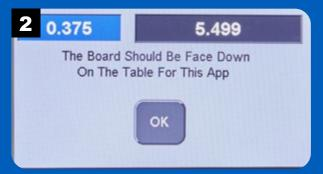
Place the workpiece with the back face on the table and one edge against the fence. Press OK. **NOTE:** Clamp a stop block to the fence to aid in positioning the workpiece for routing.
