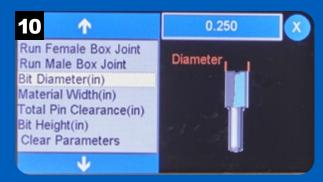
Set the bit diameter by pressing the value field in the upper right. **NOTE:** It's best to measure the actual diameter of the bit with calipers rather than rely on the stated diameter.
