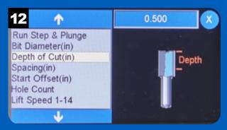
The Depth of Cut option allows you to set the depth of the dowel holes.
