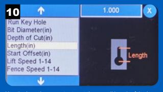
Use the Length parameter to set the overall length of the key hole slot. NOTE: The dimension entered is the center-to-center distance between the clearance hole and slot end.
