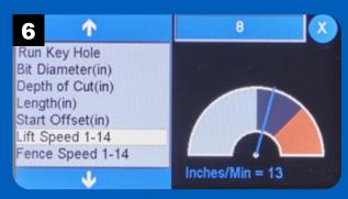
Change the speed of the router lift by entering a value between 1 and 14. The inches per minute is displayed for reference. For dense hardwoods, use a lower speed.
