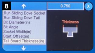
Select the Tail Board Thickness option to set the thickness of the workpiece to be routed to create the dovetail.
