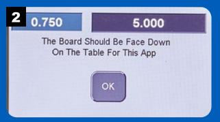
Place the workpiece face down (where the dado is to be cut). Press OK to continue.
