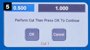
Make a pass over the router bit to create the dovetail socket and press OK.
