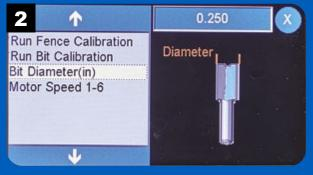
Selecting Bit Diameter from the menu displays the current value in the upper right. Press this button to change the diameter.
