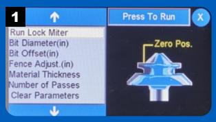
Select Run Lock Miter to start the app. Note the zero position on the lock miter router bit. This is the point of calibration using the touch plate.
