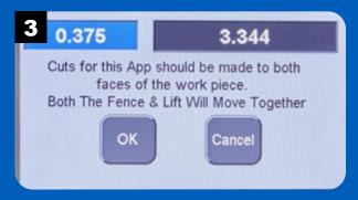
To move the lift and fence to their starting positions, press OK.
