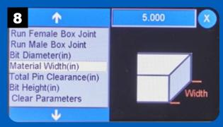
Enter the overall width of the material you're using to create the box joints by pressing the value field.
