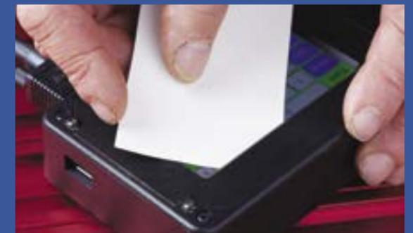
Wipe the Pendant screen with a soft cloth and remove sawdust buildup between the case and screen with a folded piece of paper.
