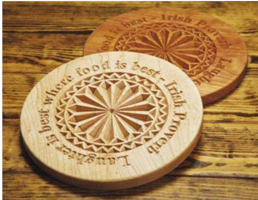
For this project, you will need a piece of solid wood that measures 12" x 12" x 3/4" thick. Hardwoods like maple or cherry work best. You will also need a waste board to place under the trivet material. Mark the center of the blank, then clamp the blank with the waste board underneath to the CNC table using the hold-down clamps, as shown in Figure 1. Install a 90° V-bit bit in the router collet and set the speed to 17,500 RPM.
