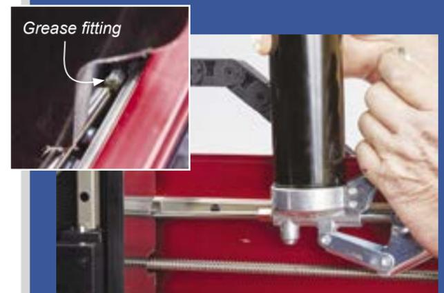
To lubricate the Z-axis bearings, you'll find the grease fittings behind the spindle mount.
