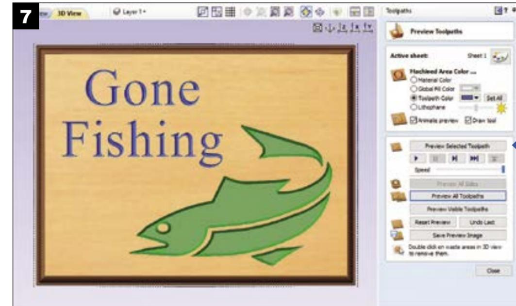
Check the toolpaths you wish to save and select the Post-Processor that matches your machine. For your Shark CNC router select the Next Wave CNC (\*.tap) post processor. The post processor converts the VCarve drawing and toolpath selections into a file that tells your
