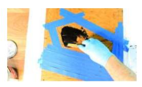
Now the next step is to fill in the inlay, the inlay will be filled in with polyester body filler with a black dye. We will mask off our graphic mix up our filler and fill in the inlay graphic area. The next step is to sand down the filler flush with the rest of the board.
